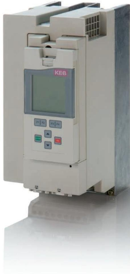
Digital operator, part no. **00F5060-1100** display and keyboard operation, plug-in module, prepared in connection with the ready-made HSP5 operator **00F5060-9000** + cable **00F50C0-2030** (3 m) / **-2100** (10 m) for external use as remote operator.
